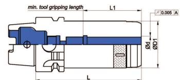
\*Special design of dust-proof extends 50% or more lifetime of tool holders. \*Caution: Excessive tightening torque will damage the chuck, nut or / and collet permanently!
