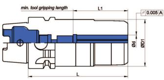
\*Special design of dust-proof extends 50% or more lifetime of tool holders. \*Caution: Excessive tightening torque will damage the chuck, nut or / and collet permanently!
